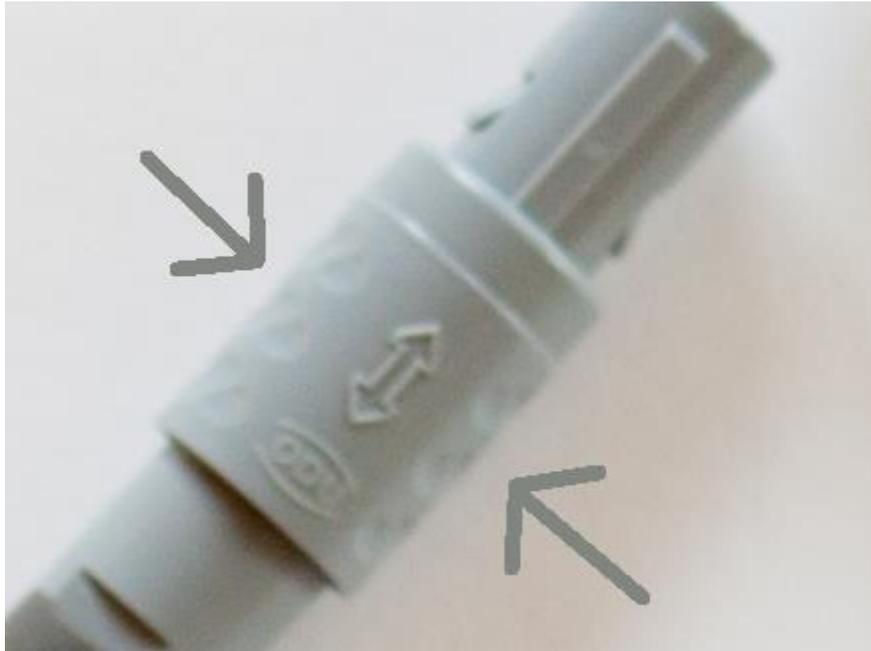
**Note:** Do not pull on the cable itself and pull only on the ODU connector as shown above.
