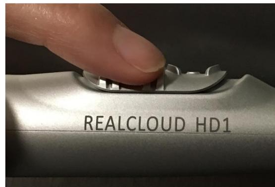
To focus the camera, move the slider forward or back until the image becomes in focus. To focus close-up, move the slider toward the tip of the handpiece; to focus further away move the slider towards the base of the handpiece.
